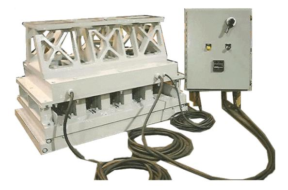
The Columbia remote temperature controller part #603712.B is designed to heat the mold shoes. Heating the mold assembly shoes prevents block material from adhering to mold shoe surfaces as block is formed in the production process. The remote temperature controller regulates the temperature of the mold shoes using temperature feedback and RTD devices.
